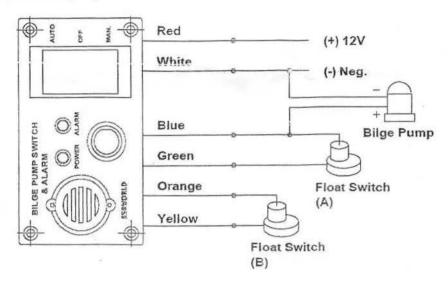
Use min #16 gauge marine grade electrical wire.
